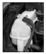
The coolant level should be at the FULL COLD mark. If it isn't, you may have a leak at the pressure cap or in the radiator hoses, heater hoses, radiator, water pump or somewhere in the cooling system.
